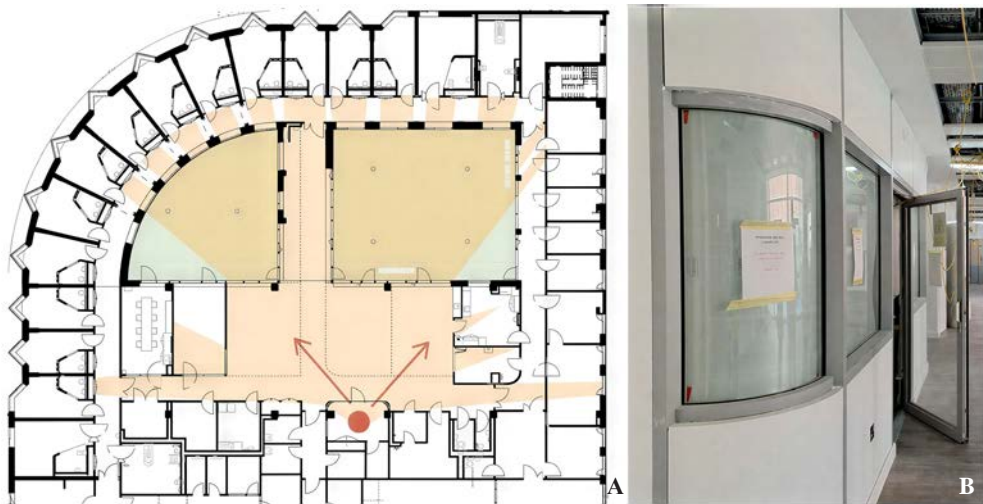
Fig. 8. Diagram of the visibility field of the ward from the nursing station (A) [C.F. Møller Architects]; nursing station as a risalit with glass corners, photo from the construction site (B) [photo: author]
